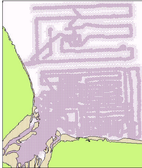
Figure 11.5. Zones around track data indicating areas where interpolation could be expected to return reliable estimated values for E1 and E2 (dark shade) and less reliable estimates (pale shade). Estimates for areas outside of these zones would be the local non-spatial average (see text).
